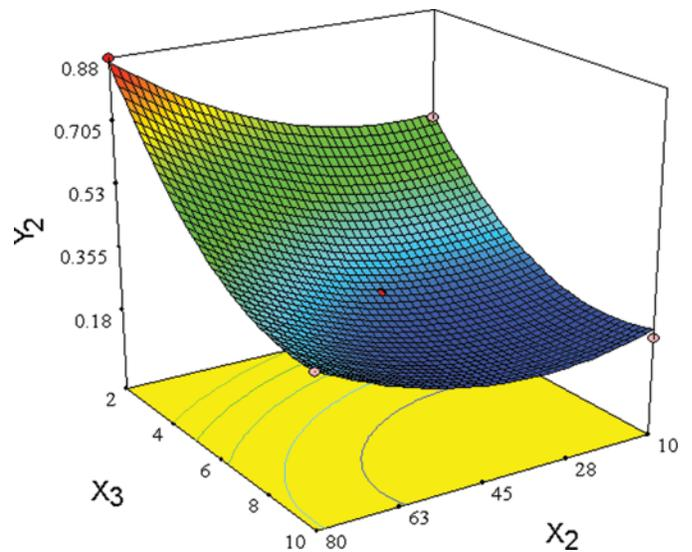
FIG. 6. Fitted surface for the PDI as a function of homogenization pressure ( $X_2$ ) and homogenization cycles ( $X_3$ ) (stirring velocity = 13000 rpm). (Figure available in color online.)
