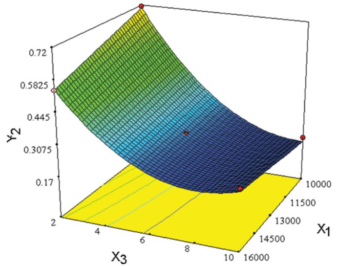
FIG. 5. Fitted surface for the PDI as a function of stirring velocity ( $X_1$ ) and homogenization cycles ( $X_3$ ) (homogenization pressure = 45 Mpa). (Figure available in color online.)
