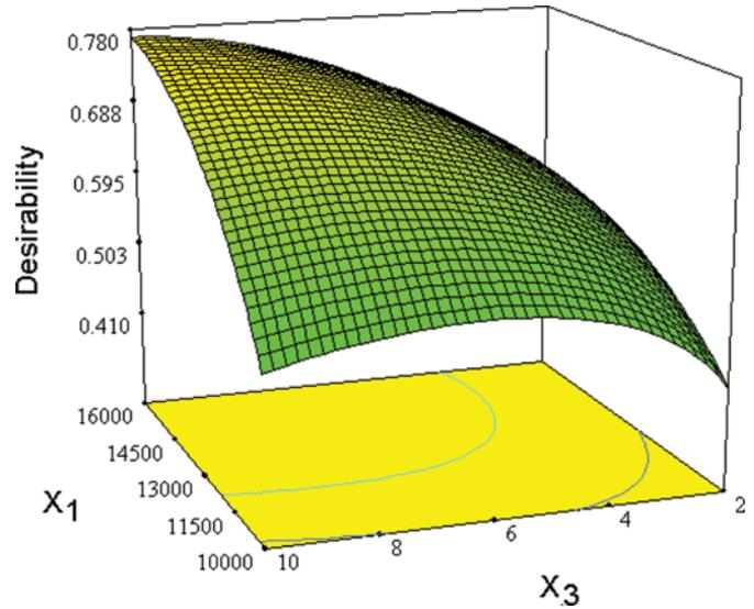
FIG. 9. Fitted surface for the desirability as a function of stirring velocity (X<sub>1</sub>) and homogenization cycles (X<sub>3</sub>) (homogenization pressure = 50 Mpa). (Figure available in color online.)
