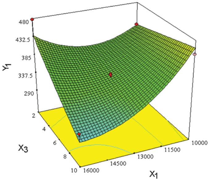
FIG. 3. Fitted surface for the particle size as a function of stirring velocity ( $X_1$ ) and homogenization cycles ( $X_3$ ) (homogenization pressure = 45 Mpa). (Figure available in color online.)
