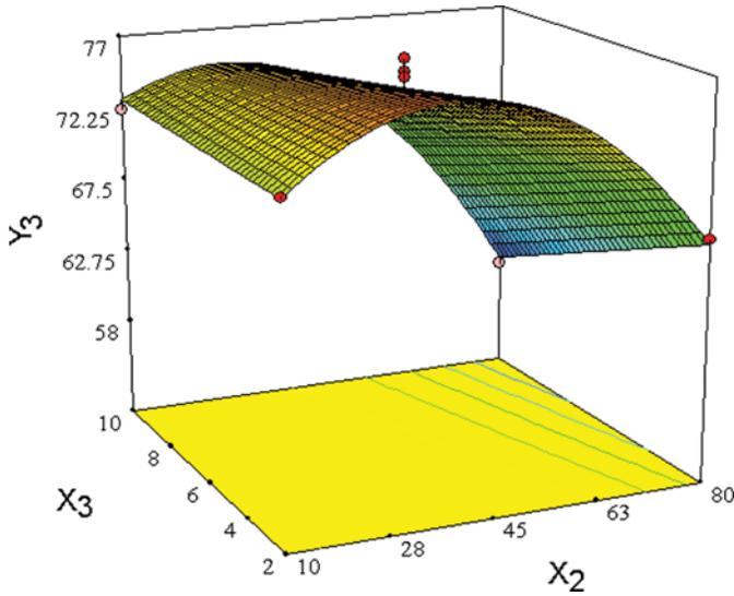
FIG. 7. Fitted surface for the entrapment efficiency (%) as a function of homogenization pressure (X<sub>2</sub>) and homogenization cycles (X<sub>3</sub>) (stirring velocity = 13000 rpm). (Figure available in color online.)
