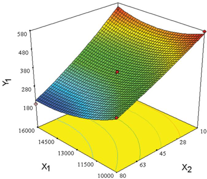
FIG. 4. Fitted surface for the particle size as a function of stirring velocity ( $X_1$ ) and homogenization pressure ( $X_2$ ) (homogenization cycles = 6). (Figure available in color online.)
