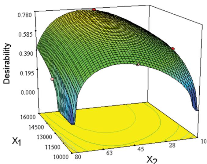
FIG. 10. Fitted surface for the desirability as a function of stirring velocity ( $X_1$ ) and homogenization pressure ( $X_2$ ) (homogenization cycles = 10). (Figure available in color online.)
