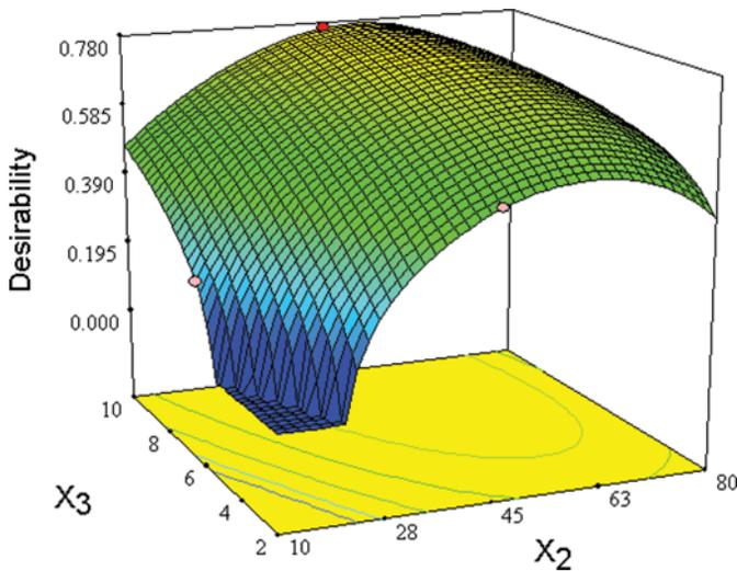
FIG. 8. Fitted surface for the desirability as a function of homogenization pressure (X<sub>2</sub>) and homogenization cycles (X<sub>3</sub>) (stirring velocity = 16000 rpm). (Figure available in color online.)
